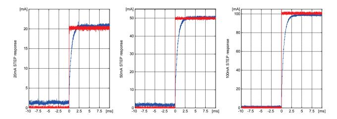
Fig. A.7: Step response for different current levels, when no current in high side
