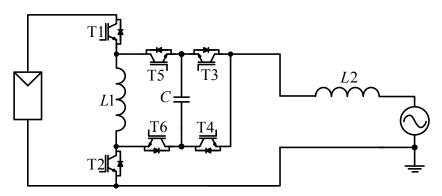
Fig. 2.16: Transformerless PV inverter topology patented by Schekulin [47].
