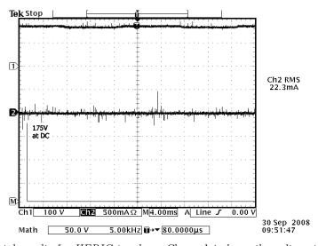
Fig. 5.17. Experimental results for HERIC topology, Channel 1 shows the voltage to ground of the DC+ terminal, Channel 2 shows the ground leakage current and Channel M shows the voltage to ground of the DC+ terminal.
