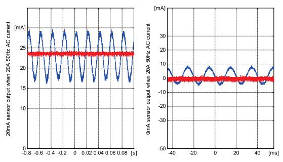
Fig. A.9: Test results for 20 mA and 0 mA(zero) leakage current,
