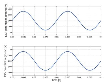
Fig. 3.17: Voltage to ground for both terminals of the PV array for the single-phase H5 topology (output filter according to case 2).
