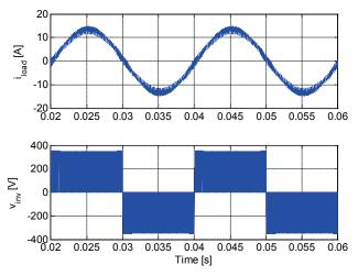
Fig. 5.4. H-Bridge topology with Unipolar PWM, load current and inverter output voltage.
