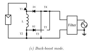
Fig. 2.15: Three different operation modes of the flying inductor inverter.
