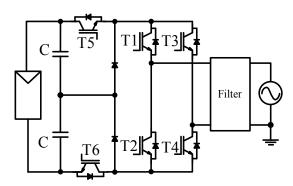
Fig. 2.20: Transformerless topology by Gonzales et al. [53].
