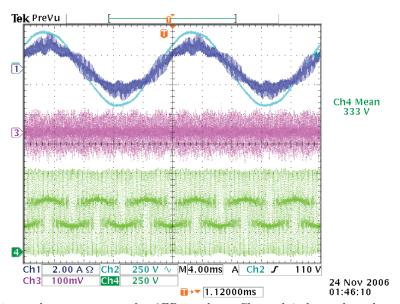
Fig. 3.23: Experimental measurements for 3FB topology. Channel 4 shows the voltage to ground of the DC+ terminal [250V/div].
