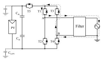
Fig. 3.16: Path of the current in case of the zero voltage vector, for positive load current (H5-SMA).
