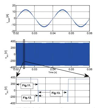
$Fig.\ 5.13.\ HB\text{-}ZVR\ load\ current\ and\ inverter\ output\ voltage.$
