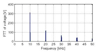
Fig. 3.6: Simulation results, FFT of voltage to ground having a bipolar PWM (grid side filter is according to case 1 from Fig. 3.2).
