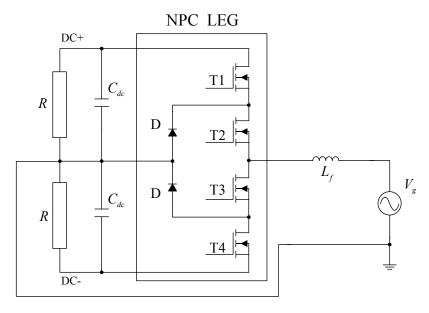
Fig. 4.9: Electrical circuit of the experimental setup using the NPC rectifier.
