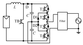
Fig. 2.17: Neutral point diode clamped inverter [37], [49] and [50].
