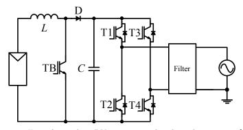
Fig. 2.8: Transformerless PV inverter with voltage boost stage [37].
