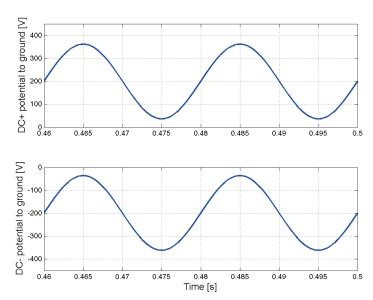
Fig. 3.7: Simulation results, voltage to ground for both terminals of the PV array with bipolar PWM (grid side filter is according to case 2 Fig. 3.3).
