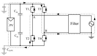
Fig. 3.5: T2-T3 turned-ON, for -V<sub>DC</sub> output voltage.
