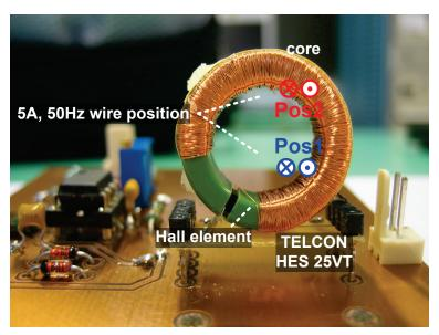
Fig. A.10: Telcon HES 25VT sensor, without the plastic casing
