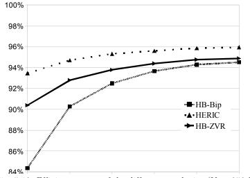
Fig. 5.19. Efficiency curve of the different topologies ( $V_{dc}$ =350 V).
