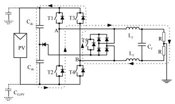
Fig. 5.11. HB-ZVR topology, dead-time between turn-OFF of T1-T4 and turn-ON of T5, during positive half-wave.
