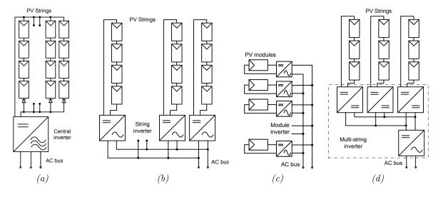
Fig. 2.2: Different grid-connected PV inverter structures: Central inverter (a); String inverter (b);
