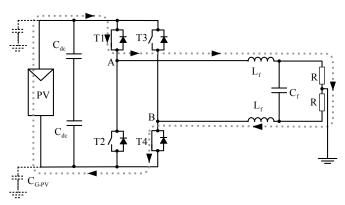
Fig. 5.2. H-Bridge topology with Unipolar PWM, active vector applied to load, using T1-T4 for positive voltage.
