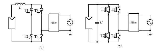
Fig. 2.7: Typical single-phase PV inverter, past and present topology, showing a line commutated inverter(a) and an H-Bridge (force commutated) inverter (b) [36].
