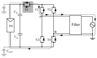
Fig. 3.15: Path of the current in case of the positive voltage vector, for positive load current (H5-SMA).
