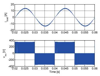
Fig. 5.8. HERIC topology, load current and inverter output voltage.
