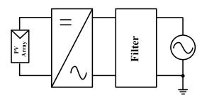
Fig. 2.4: Grid connected PV system with transformerless inverter.
