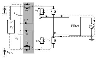
Fig. 3.18: Single-phase topology with DC decoupling used for transformerless PV systems.
