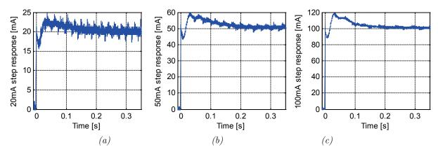
Fig. A.3 LEM CT 0.2-P step response for 20mA (a), 50mA (b) and 100mA (c) leakage current and with 20A current in high power side
