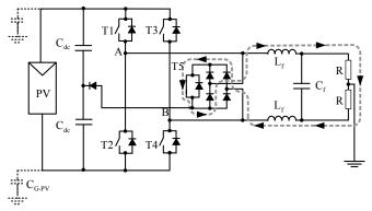
Fig. 5.12. HB-ZVR topology, zero voltage applied to load, using T5, during positive half-wave.
