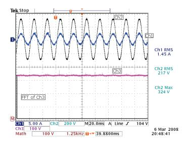
Fig. 4.7. Experimental results for single-phase NPC inverter: Channel 1: grid current [5A/div]; Channel 2: grid voltage [200 V/div]; Channel 3: voltage between DC+ terminal and ground [100 V/div]; Channel M: FFT of Channel 3 [100 V/div and 1.25 kHz/div].
