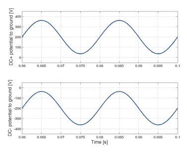
Fig. 3.19: Voltage to ground for both terminals of the PV array (topology with DC decoupling; output filter according to case 2).
