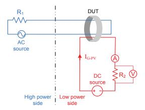
Fig. A.1 Laboratory setup for testing the step response of the sensors
