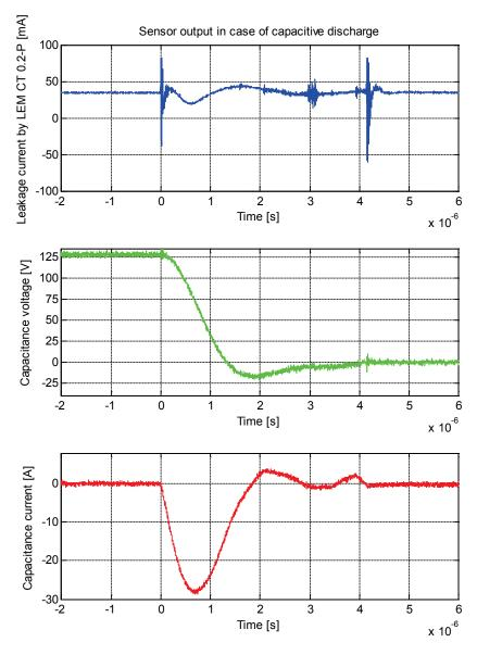
Fig. A.6: Capacitive discharge test
