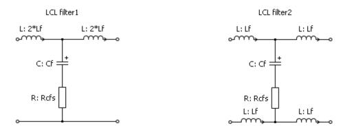
Fig. 3.2: LCL filter configuration (case 1).
