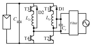
Fig. 2.13: Four-switch resonant buck-boost inverter by Wang [45].
