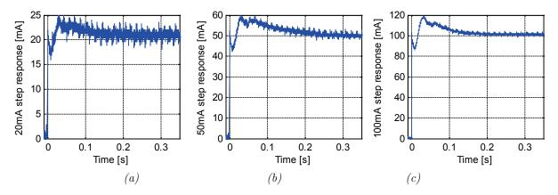
Fig. A.2 LEM CT 0.2-P step response for 20 mA (a), 50 mA (b) and 100 mA (c) leakage current and with no current in high power side
