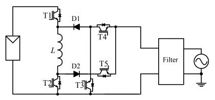
Fig. 2.14: Flying inductor inverter[46].
