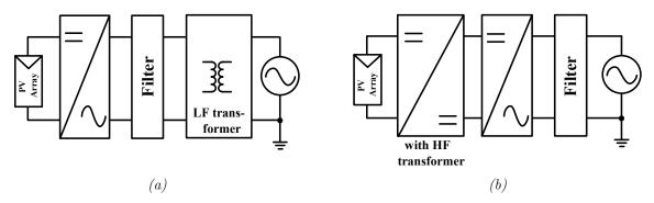
Fig. 2.3: Grid-connected PV system using an inverter with galvanic isolation: grid-side low-frequency
