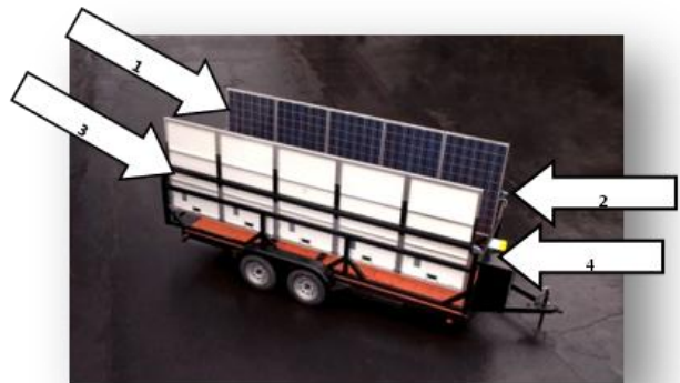
Figure 3 The four locations of the spring-loaded, locking pins
