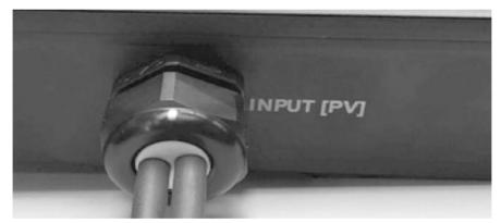
2. Attach the INPUT [PV] connectors to positive and negative connections of the PV string.
