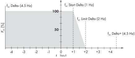
Figure 1: Operating principle of FSPC
