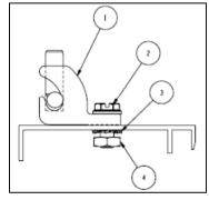
Figure 8: Grounding Lug with Nut: Grounding Diagram
