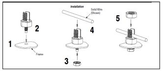
Figure 6: SolKlamp Grounding Bolt Diagram
