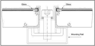
Figure 2: Clamp Mounting Example Diagram
