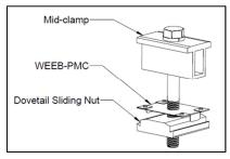
Figure 10: WEEB-PMC Assembly
