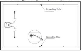
Figure 3: Grounding Hole Location
