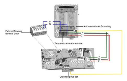
Figure 30: Connecting to the auto-transformer
