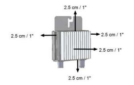
Figure 2: Power optimizer clearance
