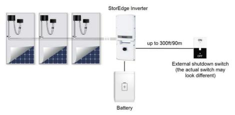
Figure 49: System connected to an external shutdown switch
