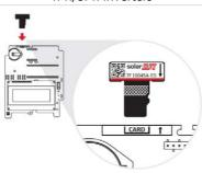
Figure 43: Inserting the upgrade card
