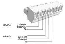
Figure 40: RS485 terminal block
