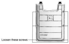
Figure 45: Opening the StorEdge Connection Unit cover
