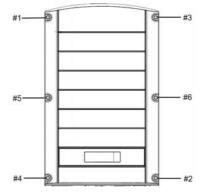
Figure 19: Tightening order of the screws
