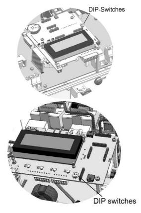
Figure 42: RS485 termination switch
