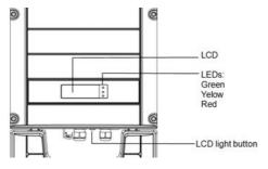
Figure 9: Inverter front view
