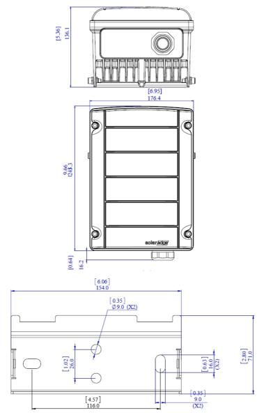
Figure 52: Auto-transformer dimensions (mm [in])
