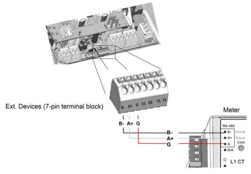
Figure 29: Connection to a meter
