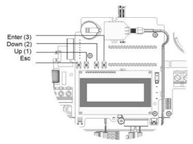
Figure 32: LCD Internal menu buttons
