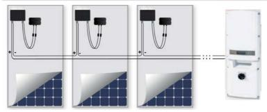
Figure 7: Power optimizers connected in series
