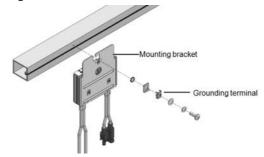
Figure 5: Power optimizer grounding terminal
