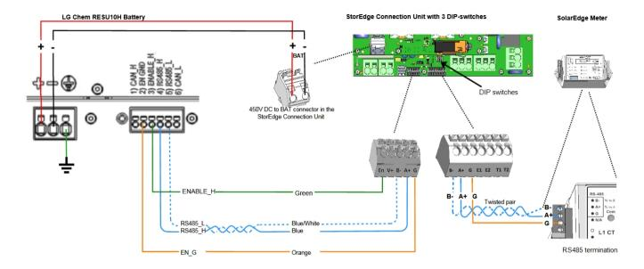
Figure 25: Connections to LG Chem RESU10H battery (StorEdge Connection Unit with three DIP-switches)
