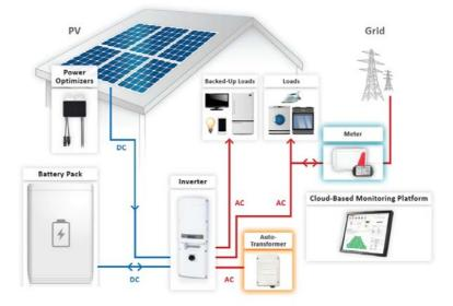
Figure 1: StorEdge system components
