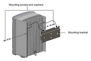
Figure 16: Installing the auto-transformer
