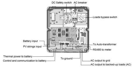
The following figure shows the connections in the StorEdge Connection Unit:
