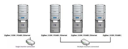
Figure 35: Example of Ethernet connection
