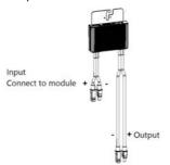
Figure 6: Power optimizer connectors
