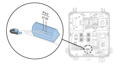
Figure 50: External shutdown switch connection
