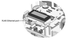
Figure 38: The RJ45 Ethernet connection
