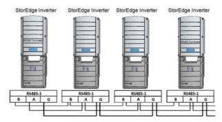
Figure 41: Connecting the inverters in a chain
