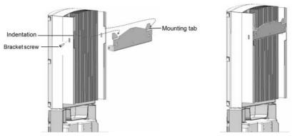
Figure 13: Hanging the inverter on the bracket
