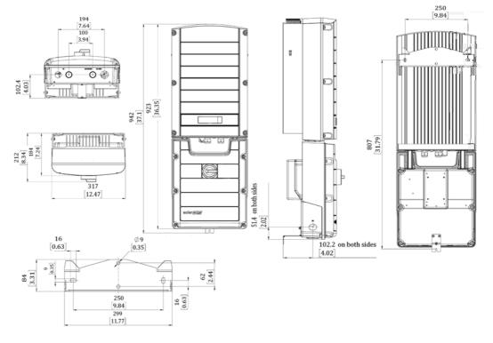
Figure 51: Inverter dimensions
