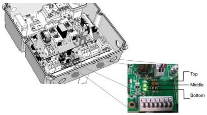
Figure 44: StorEdge Connection Unit LEDs
