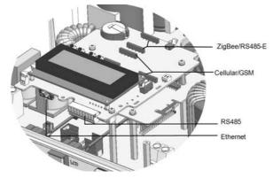
Figure 34: Internal connectors
