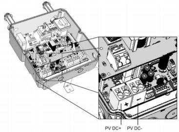
Figure 24: PV connection
