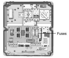
Figure 48: StorEdge Connection Unit fuses
