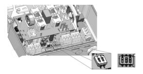
Figure 28: StorEdge Connection Unit DIP switches
