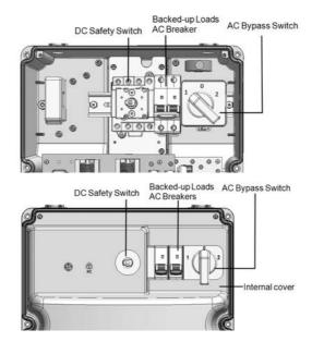
Figure 11: StorEdge Connection Unit with and without internal cover
