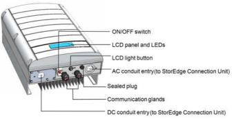
Figure 8: Inverter Interfaces
