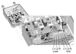
Figure 31: Connection to grid, backed-up loads
