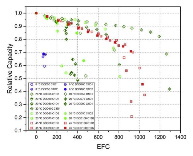
Lithium batteries lose their capacity as they age. Both Lithium and Lead Acid batteries lose cycles at higher temperatures. Assuming 20C temperature and 50% DoD, Lithium capacity will drop between 0.5% and 1.5% per month. Suggesting 8 to 12 year life span when used.
