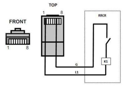
Fig.13 Inverter – RRCR Connection
