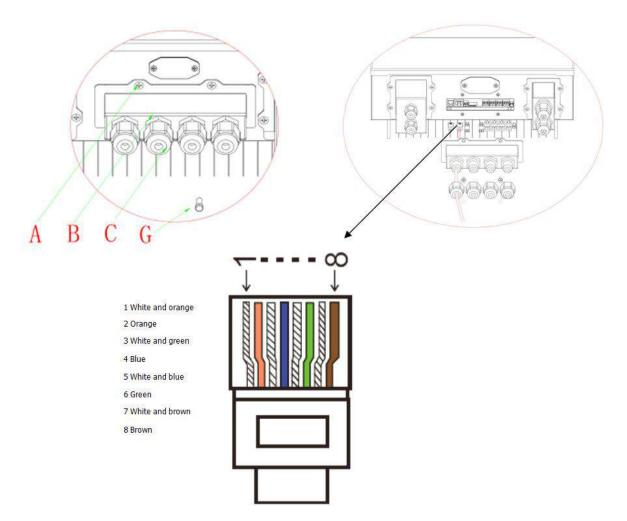
Fig. 11 Inverter logic interface connection
