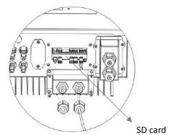
**Step 2** Press the SD card and take it out. Insert the SD card into a micro-SD card reader, then insert micro-SD card reader into a PC; (NOTE: micro-SD card reader & PC are not provided by SOFARSOLAR).
