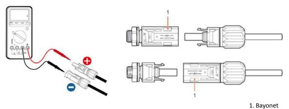
Fig. 9 Connect PV connectors
