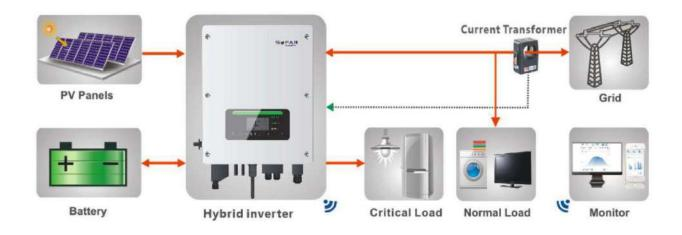
Fig. 1 HYD-ES inverter schematic diagram
