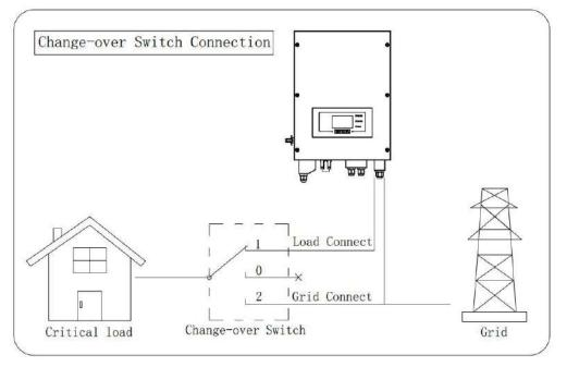
Fig. 18 Change-over Switch connections
