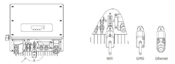
The operation information (generated energy, alert, operation status) of the inverter can be transferred to PC or uploaded to the server via WiFi /GPRS/ Ethernet. You can register on the website. http://www.solarmanpv.com/portal/Register/Regi\_Pub.aspx
