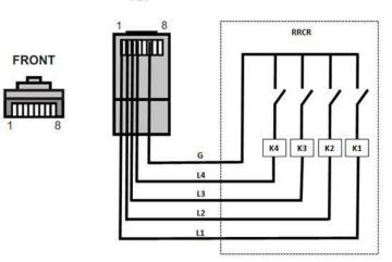
Fig.12 Inverter – RRCR Connection
