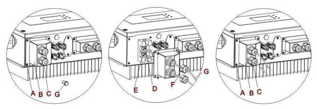
Fig. 6 Battery connection (Measure battery wires polarity/voltage before connection)
