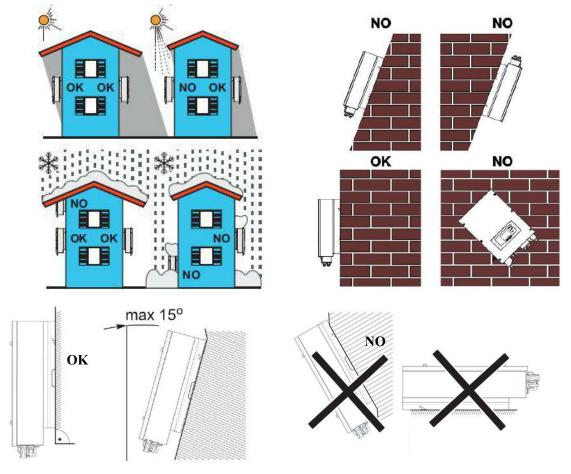
Fig. 4 Installation Position of HYD-ES inverter
