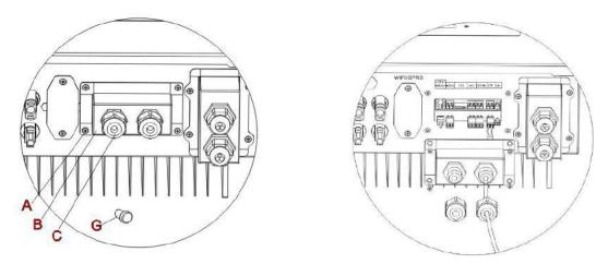
Fig. 15 CT / CAN / RS485 / NTC connection
