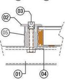
Fig. 4e: CAMO hidden end clamp. Clamp slide into rail channel and the bonding pins contacts the module flange edge.
