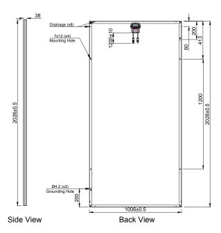
Fig. 3b: Mechanical drawing of the SIL NT and SIL MT modules showing the mounting holes, the drainage holes, and the ground connection holes.
