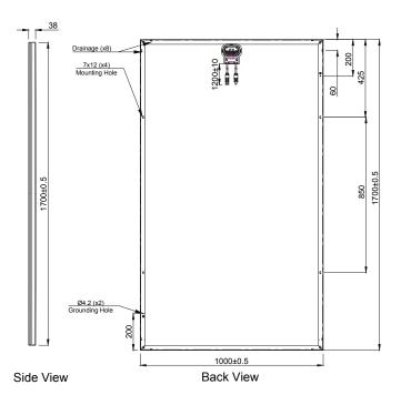
Fig. 3a: Mechanical drawing of the SIL NL, SIL ML, SIL HL and SIL XL modules showing the mounting holes, the drainage holes, and the ground connection holes.
