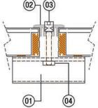
Fig. 4c: modules attached to supporting structure - side view
