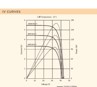
Current, Power vs. Voltage Characteristics \_\_\_\_\_ Power vs. Voltage
