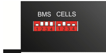
Figure 3: Address and cell selection DIP Switches.
