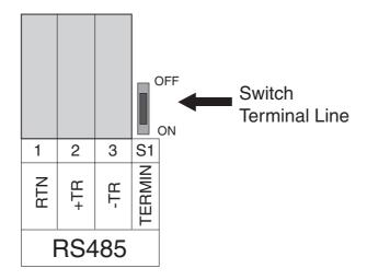
Fig.17: The RS-485 serial link terminal blocks
