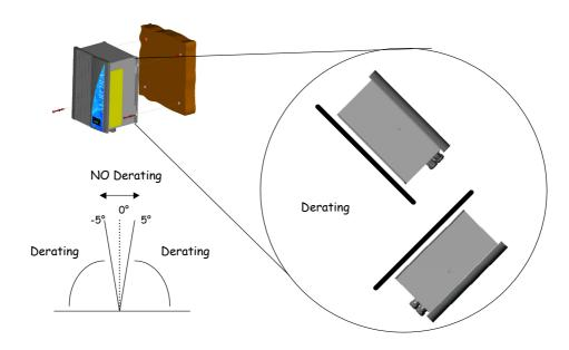
Fig.8 Inverter tilted mounting
