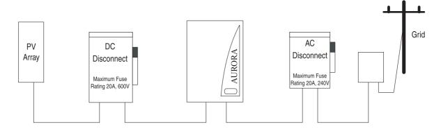
Wire in accordance with NEC Section 690 and applicable local codes
