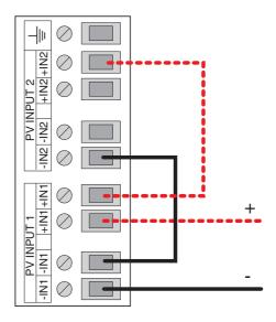
Fig.14: Paralleling the two input sections
