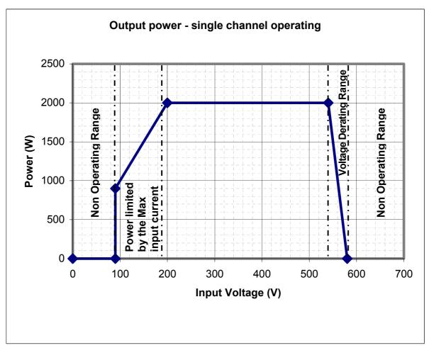
The two above cases, originating a power derating, can also occur at the same time, but the power derating will always correspond to the lowest value read.
