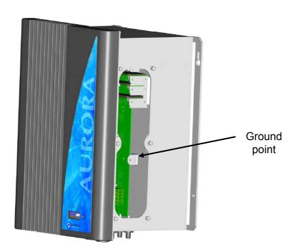
Fig.13: Location of Main Ground PE Screw
