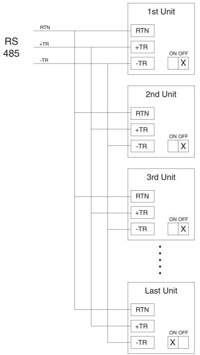
Fig.18 Multiple units connection
