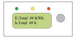
✓ Sixth screen: Time during which the unit exported energy to the grid, and number of times that unit connected to the grid.
