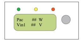
✓ Fourth screen: Output power and Voltage Input on the second photovoltaic array
