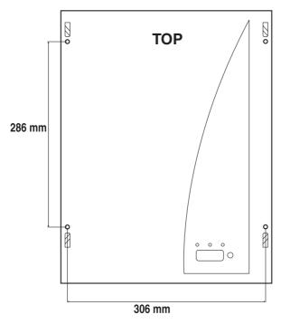
Fig.6 Wall mounting diagram
