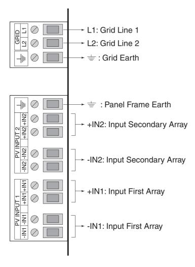
Fig 12: Screw terminal blocks
