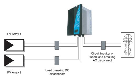
Fig.3 Simplified diagram of a photovoltaic system
