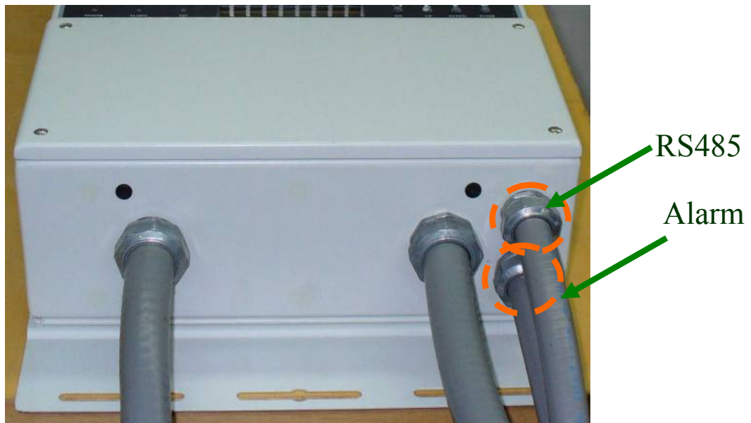
Fig.23a - Holes for cables necessary for RS-485 port connection or wiring for RJ12 connector connection (without the switch box).
