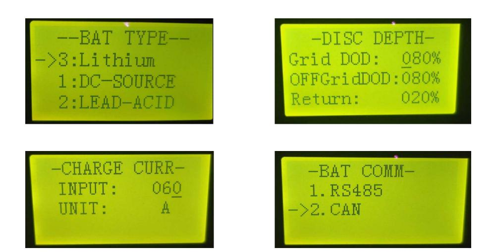
The recommended charging current is arround 60A(5kWh) and 80A (10kWh)
