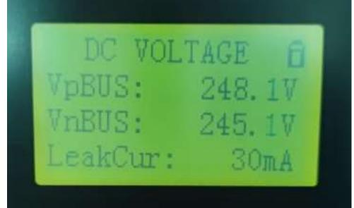
The DC BUS voltage is the DC bus voltage inside the inverter (the DC bus voltage after the PV input is tracked and transformed by the MPPT) Vp BUS (BUS peak voltage) Vn BUS (BUS normal voltage)
