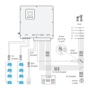
The CT arrow points to the grid, otherwise the inverter will display wrong data or the machine will not work properly.
