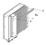
**Step 3**: Place the inverter on the wall-mounted bracket by holding the handle on the side.
