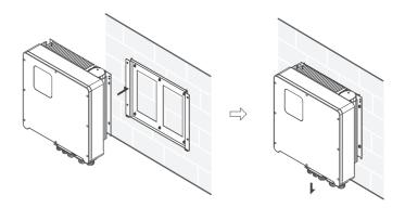
**Step 4**: Tighten the fixing screws on both sides of the inverter.
