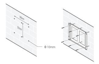
Step 2: Use the screws to fix the crossbar as shown in the figure below.
