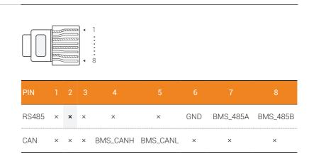
When using RS485 protocol, please note that PIN2 must be disconnected.
