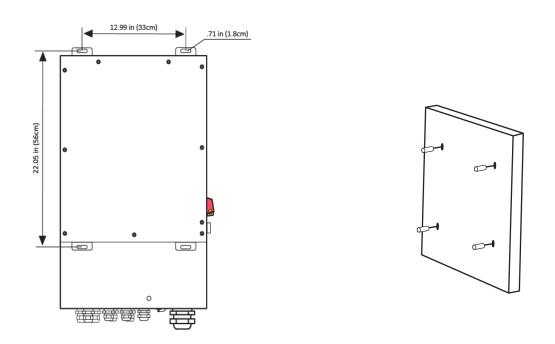
**Step 2:** Lift up the inverter and align the holes of the inverter with the expansion bolt, mount the inverter on the wall.
