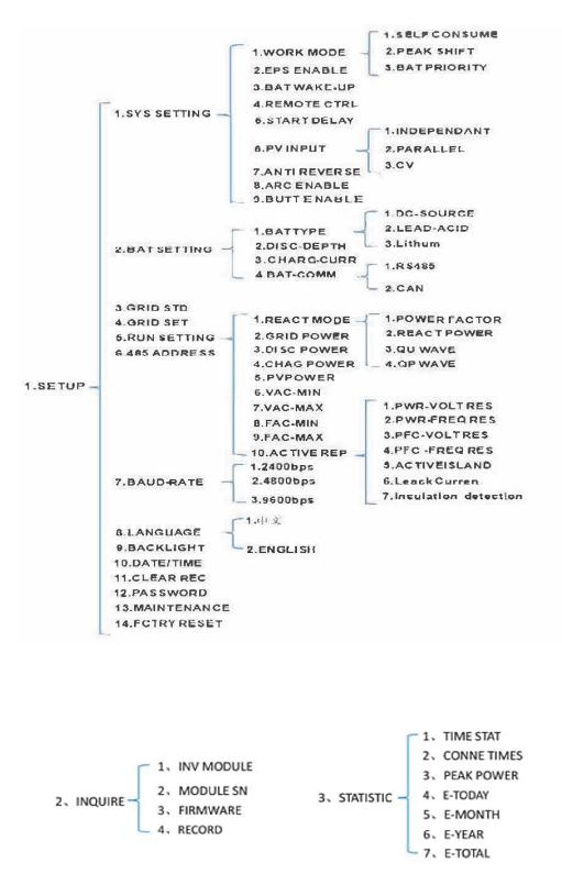
For example, before selecting the mode, you can set it up according to the local power grid.
