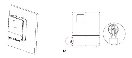
**Step 4**: Remove the cover screws by Allen Wrench and remove the cover. Remove the waterproof cover by a flat blade screwdriver. Wiring box conduit plugs, Conduit plugs are provided for 1 inch conduit fittings. If used conduit fitting is not 1 inch, an appropriate conduit adaptor should be used.
