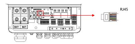
**Step2.** Insert one RJ45 side of the cable into Meter port inside of inverter and the other side into BMS-485port of the meter.
