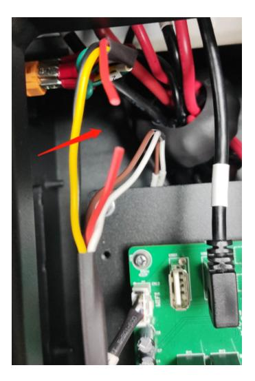
(2) Step 2: Connect the Live Line to the following male connector.
