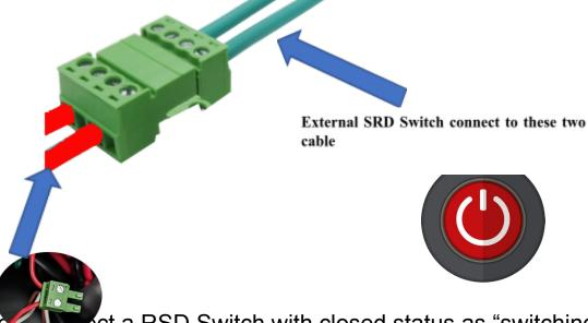
Note: plece a RSD Switch with closed status as "switching on condition". The system will keep on normal working condition if the External RSD Switch stay in closed status, while the Rapid Shut Down will take action while the External RSD Switch is in the status of opening.
