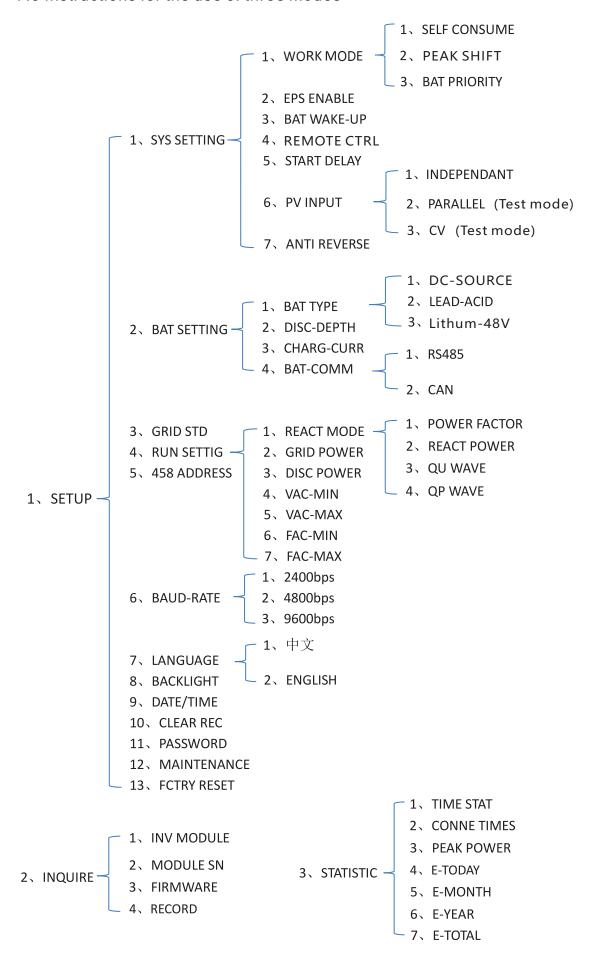
For example,Before selecting the mode, you can set it up ac cording to the local power grid, PV input mode and battery type.
