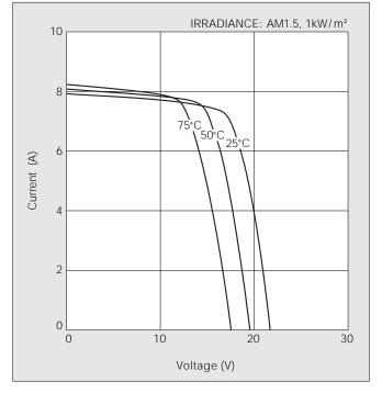
Current-Voltage characteristics of Photovoltaic Module KC125GT at various irradiance levels
