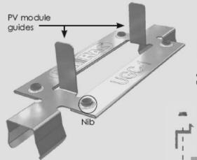
Figure 1. Slide UGC-1 grounding clip into top mounting slot of rail. Torque modules in place on top of clip. Nibs will penetrate rail anodization and create grounding path through rail.
