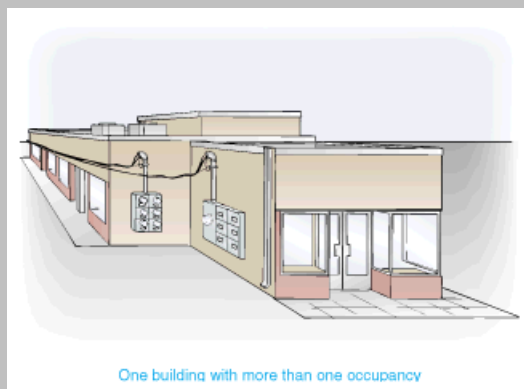
Exhibit 230.2 Two services. Two service drops supplying two services installed at separate locations for a building where there is no available space for service equipment accessible to all occupants. Maximum of six service disconnecting means for each service.
