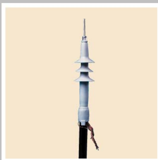
Exhibit 310.2 A one-piece, premolded stress-relief cone for indoor cable terminations of up to 35 kV phase-to-phase.
