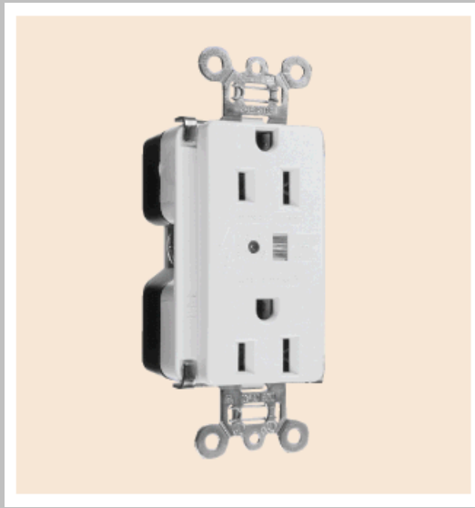
Exhibit 285.2 A TVSS as an integral component of a receptacle, providing local point-of-use protection of equipment when transient events occur within the facility. (Courtesy of Pass & Seymour/ Legrand®)
