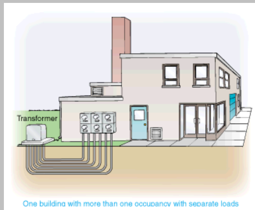
Exhibit 230.7 One service. One service lateral consisting of six sets of conductors 1/0 AWG or larger, terminating in a single service equipment enclosure with maximum of six service disconnecting means.
