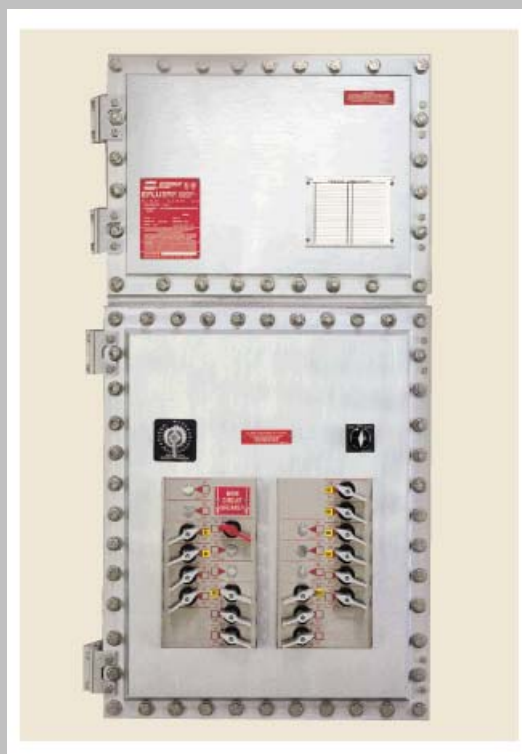
Exhibit 502.4 A dust-ignitionproof panelboard for use in Class II, Group E, F, and G locations. (Courtesy of Cooper Crouse-Hinds)
