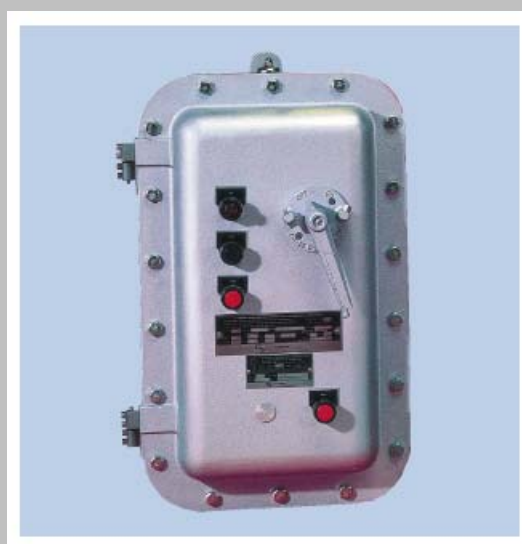
Exhibit 501.16 A magnetic motor starter for use in a Class I, Group D location. Note the number of securing bolts and the width of the flange. (Courtesy of O-Z/Gedney, a division of EGS Electrical Group)
