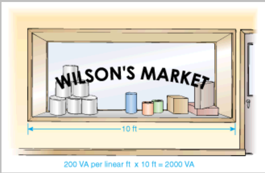
Exhibit 220.1 An example of the linear-foot load calculation for branch circuits serving a show window.
