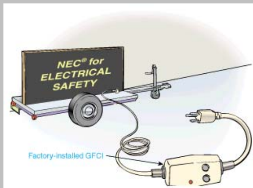
Exhibit 600.4 A factory-installed GFCI device located in the power supply cord within 12 in. of the attachment plug.
