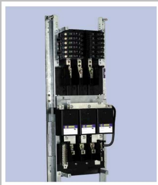
Exhibit 285.3 A TVSS mounted as an integral component of a panelboard, which minimizes conductor length between the electrical system and the TVSS. (Courtesy of Square D Co.)
