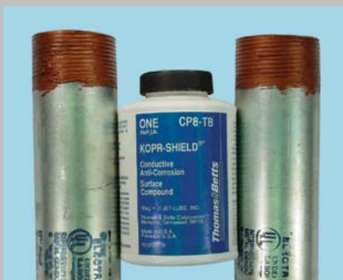
Exhibit 300.12 KOPR-Shield® (a registered trademark of Jet Lube), a conductive anti-corrosion surface compound suitable for application on field-cut conduit threads where protection from corrosion is necessary. (Courtesy of Thomas & Betts)
