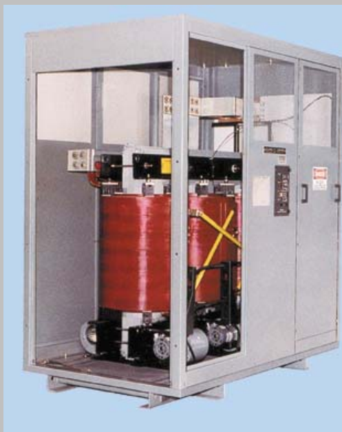
Exhibit 450.13 A dry-type transformer with a core and coil design rated at 1000 kVA, 13,800 volts to 480 volts, 3-phase, 60 Hz. (Courtesy of Square D Co.)
