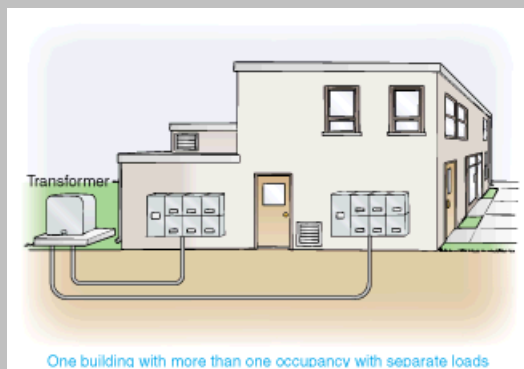
Exhibit 230.12 Two services. Two service laterals supplying two service equipment enclosures installed at separate locations, each enclosure with a maximum of six service disconnecting means.
