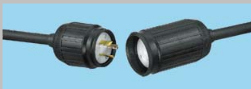
Exhibit 590.3 A watertight plug and connector used to prevent tripping of GFCI protective devices in wet or damp weather. (Courtesy of Hubbell, Inc.)
