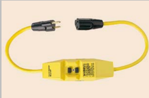
Exhibit 590.1 A raintight GFCI with open neutral protection that is designed for use on the line end of a flexible cord. (Courtesy of Pass & Seymour/Legrand®)
