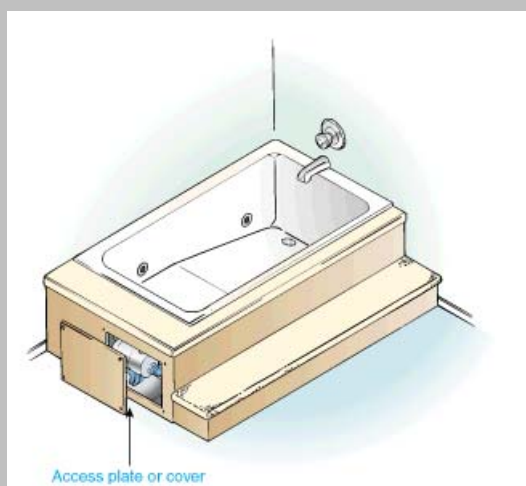
Exhibit 680.19 Access plate for hydromassage tub electrical equipment, located as described in 680.73.
