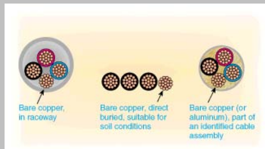
Exhibit 230.23 Bare grounded service-lateral and service-entrance conductors for underground locations.
