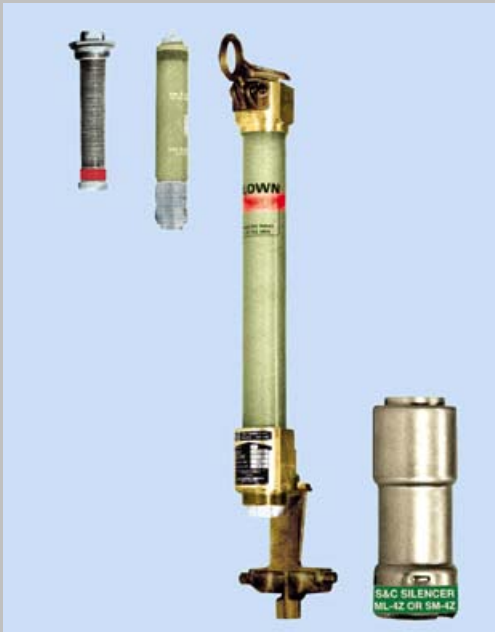
Exhibit 490.2 Components of the indoor solid-material (SM) power fuseholder (boric-acid arc-extinguishing type) with a 14.4 kV, 400E-ampere maximum, 40,000-ampere rms asymmetrical interrupting rating. Shown here are the spring and cable assembly, refill unit, holder, and snuffer. (Courtesy of S&C Electric Co.)
