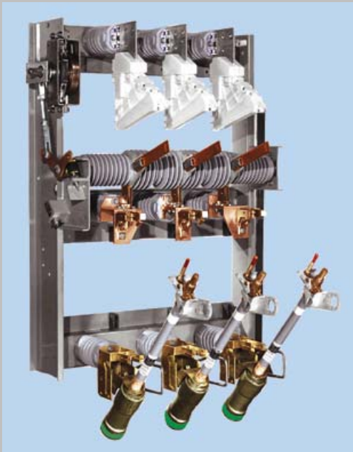
Exhibit 490.1 Group-operated interrupter-switch and powerfuse combination rated at 13.8 kV, 600 amperes continuous and interrupting, 40,000 amperes momentary, 40,000 amperes fault closing. (Courtesy of S&C Electric Co.)
