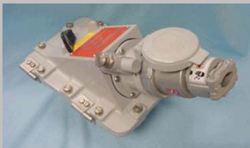
Exhibit 501.22 A receptacle and attachment plug of the explosionproof type with an interlocking switch. The switch must be in the off position before the attachment plug can be removed. (Courtesy of Appleton Electric Co., EGS Electrical Group)
