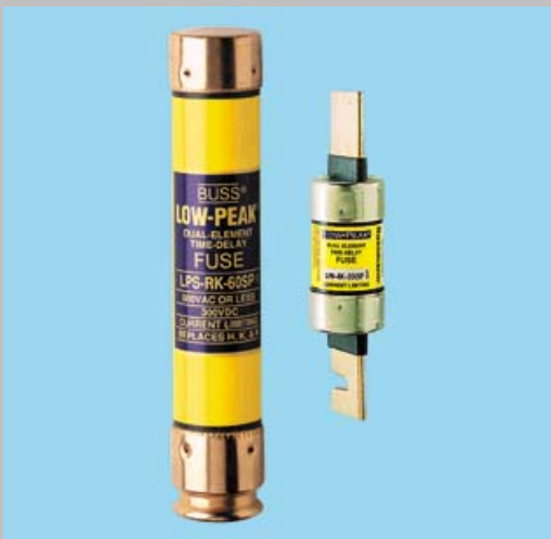
Exhibit 240.1 Class R current-limiting fuses with rejection feature to prohibit the installation of non–current-limiting fuses. (Courtesy of Bussmann Division, Cooper Industries)
