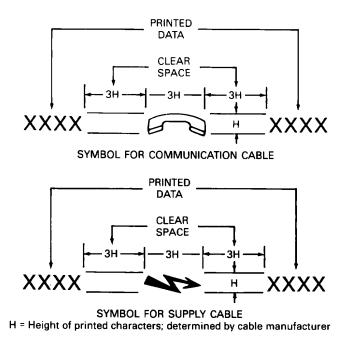
Figure 350-1—Symbols for identification of buried cables
