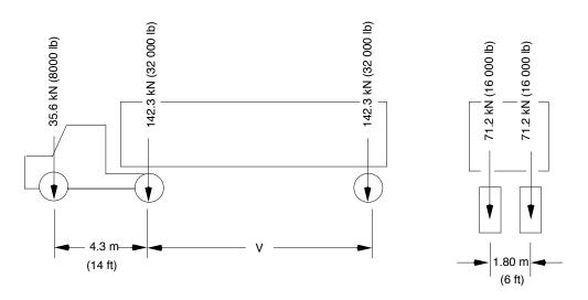
V = Variable spacing, 4.3 m to 9.0 m (14 ft to 30 ft), inclusive. Spacing to be used is that which results in vertical and lateral structure loading that produces the maximum shear and bending moments in the structure.
