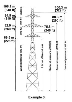
The structure wind pressure (uniformly distributed over WS#1) assuming 40 m/s (90 mph), I and  $C_d$  equal 1.0:
