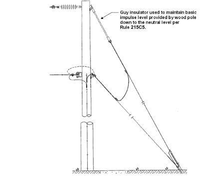
Figure 279-1—Insulator used for BIL insulation
