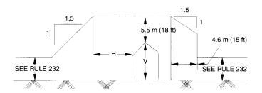
V = HEIGHT OF HIGHEST FILLING OR PROBING PORT ON GRAIN BIN H = V + 5.5 m (18 ft)
