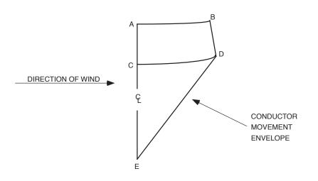
Figure 233-2—Conductor movement envelope
