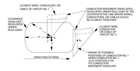
*NOTE:* In this illustration, Conductor No. 2 is closest at position  $X_2$  to Conductor No. 1, where the latter is at position  $X_1$ .
