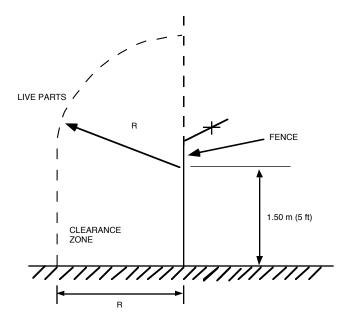
Figure 110-1—Safety clearance to electric supply station fences
