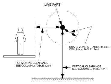
Figure 124-1—Clearance from live parts
