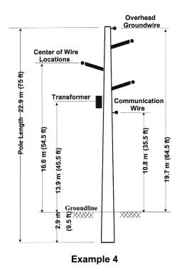
The wire wind pressure, assuming 40 m/s (90 mph), I and  $C_d$  equal 1.0, and the table values for  $k_z$  and  $G_{RF}$ , is
