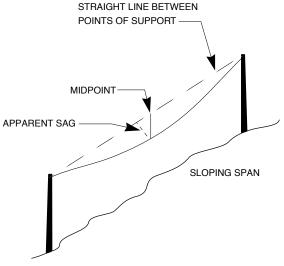
Figure D-1—Sag and apparent sag
