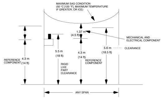
CONDITION-CLEARANCE OF OPEN SUPPLY CONDUCTORS, 750 V-22 kV, ABOVE ROADS CLEARANCE (5.6 m [18.5 ft])= REFERENCE COMPONENT (4.3 m [14 ft]) + MECHANICAL AND ELECTRICAL COMPONENT (1.37 m [4.5 ft])
