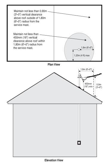
Figure 234-2—Clearances of service drop terminating on support mast
