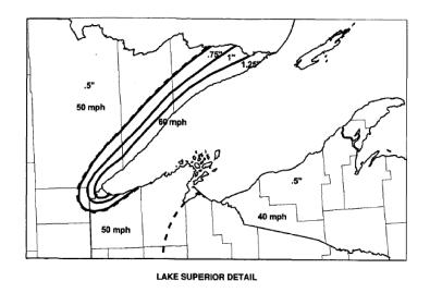
Figure 250-3(c)—Uniform ice thickness with concurrent wind
