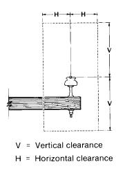
Figure 235-1—Clearance diagram for energized conductor
