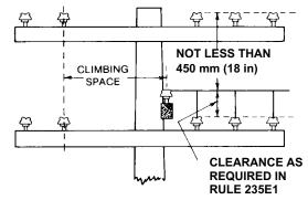
Figure 237-1—Obstruction of working space by buckarm
