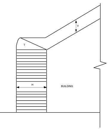
Figure 234-1(c)—Transitional clearance when H is greater than V
