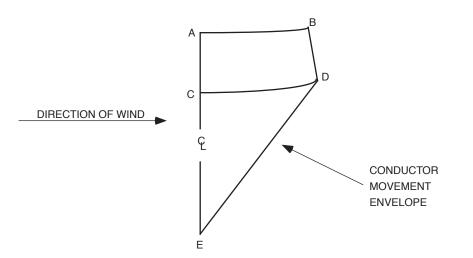
Figure 233-2—Conductor movement envelope
