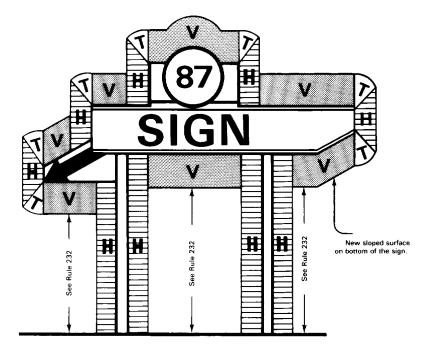
Figure 234-1(b)—Clearance diagram for other structures
