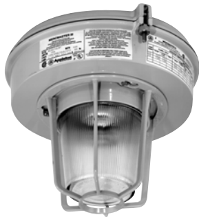
MERCMASTER III LOW PROFILE ENCLOSED AND GASKETED FIXTURE CLASS I, ZONE 2 AEx nR IIC T(X) (T number dependant on wattage and optic)
