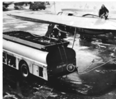
STATIC DISCHARGE REEL USED IN A FUELING OPERATION.
