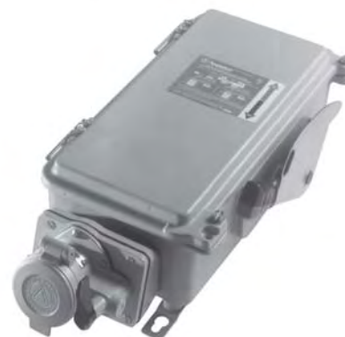
MD2SR CAST ALUMINUM RECEPTACLE WITH INTERLOCKED SWITCH AVAILABLE FUSED OR NON-FUSED. WHEN THESE RECEPTACLES ARE USED IN CLASS III, DIV. 1 OR 2 LOCATIONS, THE CONDITIONS IMPOSED BY 503.145 EXCEPTION MUST BE MET.
