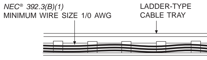
Figure 12.3 A ladder-type cable tray is permitted to support single-conductor cables, marked for use in cable trays, and multiconductor cables as listed in 392.3(A)(1).
