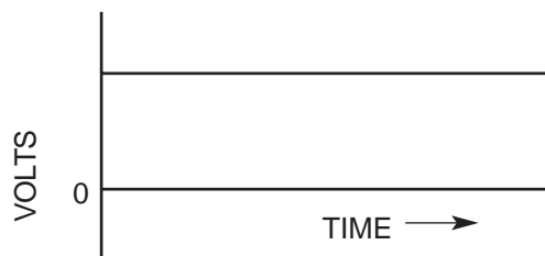
Figure 1.1 A plot of voltage in a direct current circuit over a period of time is a straight line.
