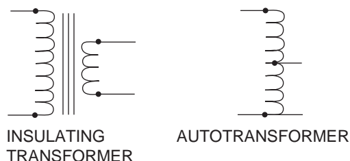
Figure 8.1 Two basic types of transformers are the insulating transformer and the autotransformer.
