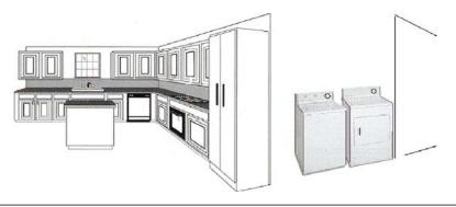
Figure 9.4 Small-appliance and laundry circuits must be included in load calculations.
