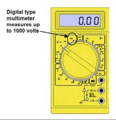
**Figure 12.7** A typical example of a multimeter that is capable of measuring voltage up 1000 V rather than a cap limit of only 600 V.
