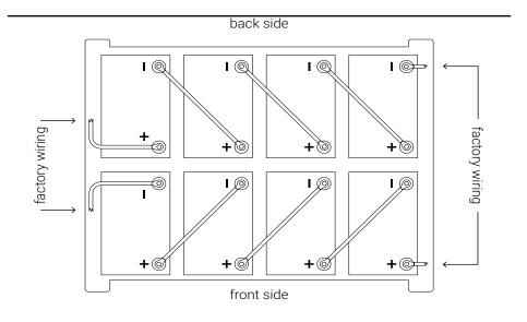
Configure and wire each level of batteries in this manner
