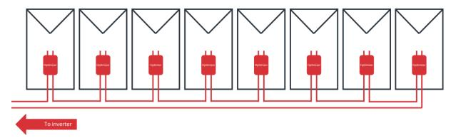
In a setup with full optimization, optimizers are installed in all modules. This type of installation is usually used to realize different orientations or roof pitches in one string. The respective optimizer automatically adjusts the current and voltage of the PV module to the current available in the string. No further adjustment or additional components are required on the part of the optimizer.
