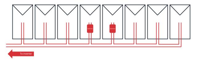
In a setup with partial optimization, optimizers are only installed in the required modules. This type of installation is usually used for small-area shading on the PV field, such as roof structures. The respective optimizer automatically adjusts the current and voltage of the PV module to the current available in the string. No further adjustment or additional components are required on the part of the optimizer.
