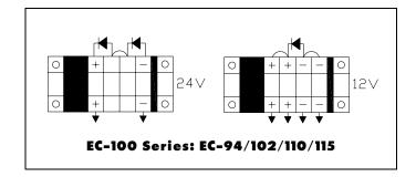
In 12-volt mode, the six terminals include two positive terminals, two negative terminals, and two spare terminals. In the 12-volt configuration, the two positive terminals are electrically equivalent, and either one can be used for power wiring; similarly for the two negative terminals. In 24-volt mode (EC-100 Series modules only), the middle two terminals should not be used for power wiring, only for jumpers and diodes.
