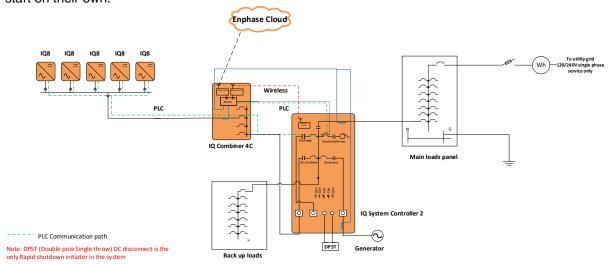
Figure 9: Enphase Energy System in Sunlight Backup configuration for IQ8-series PV microinverters. IQ System Controller 2 is installed on the load side of the main load panel with select loads backed up in a backup subpanel. The generator is wired in onto the generator port on the IQ System Controller 2.
