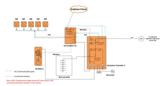
Figure 7: Enphase Energy System in Full Energy Independence configuration for IQ8-series PV microinverters. The IQ System Controller 2 is installed as a service equipment on the line-side of the main load panel and PV, IQ Battery storage system and generator are connected to the IQ System Controller 2.
