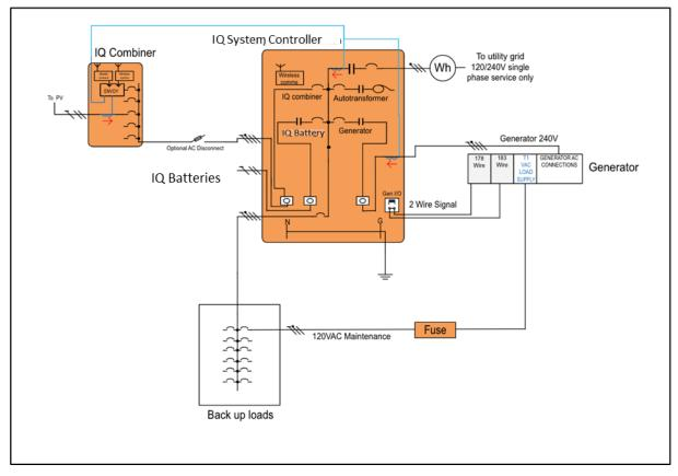
Figure 20: Generac EcoGen – Two Wire Connection
