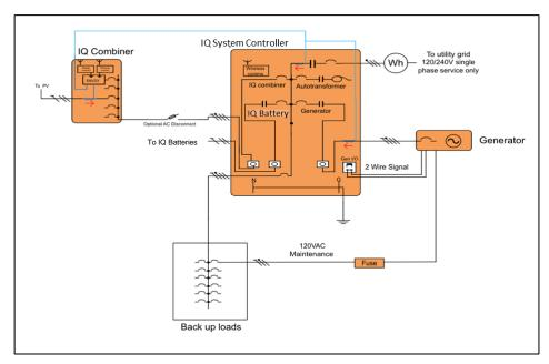
Figure 12: Generator auxiliary contact wiring for 2-wire remote start generator
