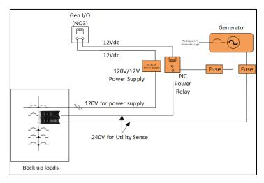
Figure 14: Utility sense wiring
