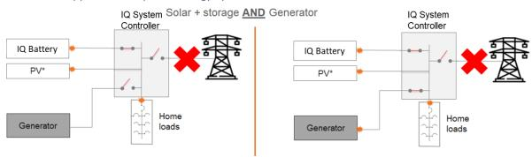
Figure 2: Enphase Energy System: Generator AND PV + storage
