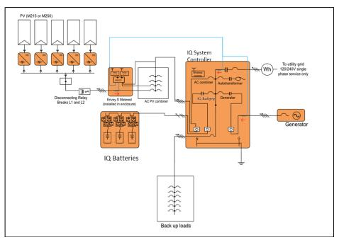
Figure 5: Enphase Energy System in Full Energy Independence configuration for M-Series PV microinverters. The IQ System Controller is installed on the line-side of the main load panel, and PV, IQ Battery storage system, and generator are connected to the IQ System Controller.
