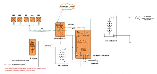
Figure 8: Enphase Energy System in Home Essentials configuration for IQ8-series PV microinverters. IQ System Controller 2 is installed on the load side of the main load panel with select loads backed up in a backup subpanel. The generator is wired in onto the generator port on the IQ System Controller 2.
