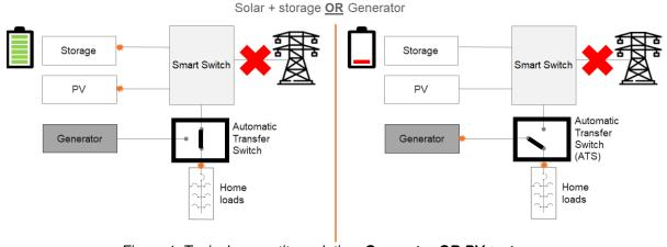
Figure 1: Typical competitor solution: **Generator** OR PV + storage
