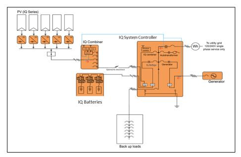
Figure 3: Enphase Energy System in Full Energy Independence configuration for IQ6/7-series PV microinverters. The IQ System Controller is installed as a service equipment on the line-side of the main load panel and PV, IQ Battery and Generator are connected to the IQ System Controller.
