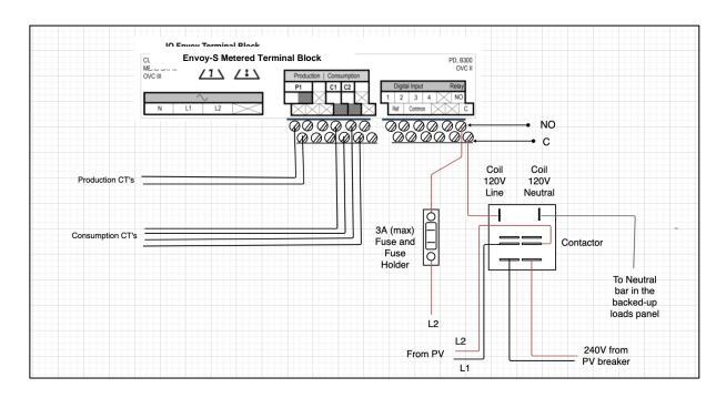
Figure 17: Wiring Envoy-S Metered for backfeed protection
