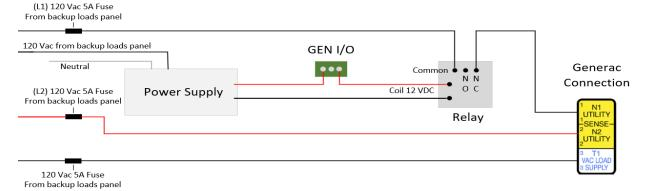
Figure 15: Wiring diagram for utility sense generator support
