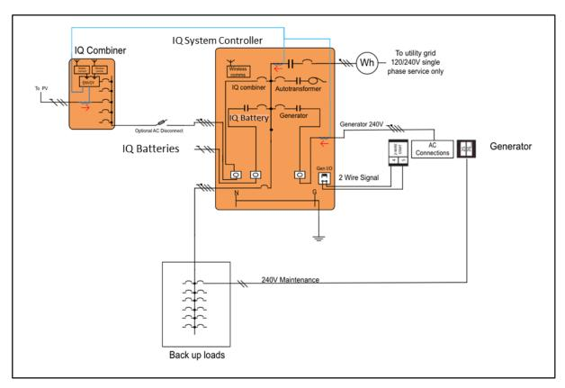
Figure 21: Briggs & Stratton - Two Wire Connection
