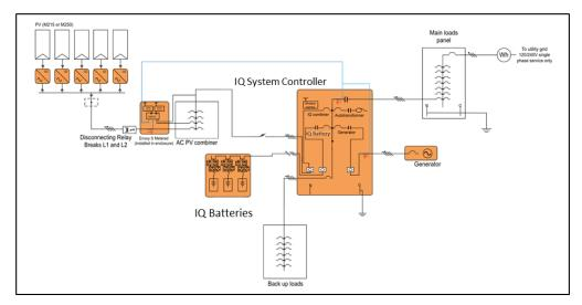
Figure 6: Enphase Energy System in Home Essentials configuration for M-Series PV microinverters. IQ System Controller is installed on the load side of the main load panel with select loads backed up in a backup subpanel. The generator is wired in onto the generator port on the IQ System Controller.
