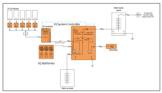
Figure 4: Enphase Energy System in Home Essentials configuration for IQ6/7-series PV microinverters. IQ System Controller is installed on the load side of the main load panel with select loads backed up in a backup subpanel. The generator is wired in onto the generator port on the IQ System Controller.
