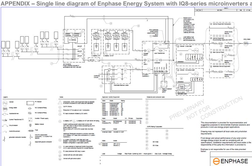
APPENDIX – Single line diagram of Enphase Energy System with IQ8-series microinverters and generator
