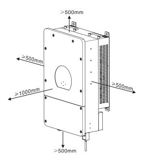
For proper air circulation to dissipate heat, allow a clearance of approx. 50cm to the side and approx.50cm above and below the unit.And 100cm to the front.
