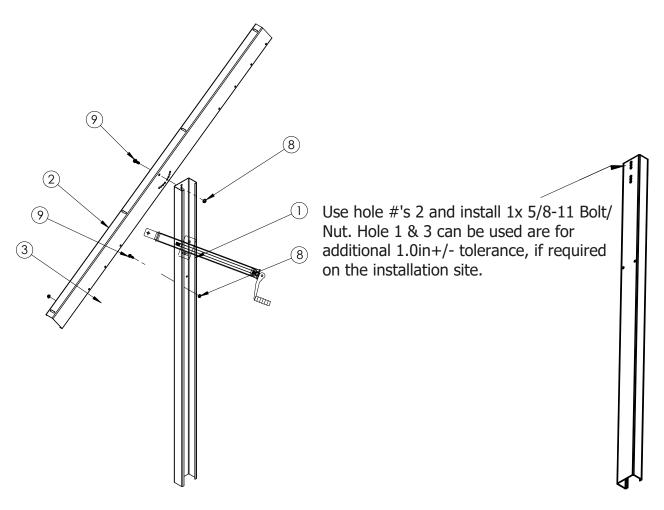
STEP 1: Install TRUSS to the C-Channel Post with 2x 5/8-11 x 1 1/2in Bolts/Nuts.
