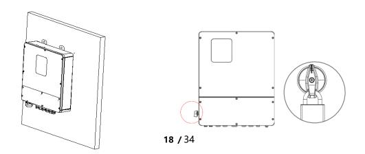
**Step 4**: Remove the cover screws by Allen Wrench and remove the cover. Remove the waterproof cover by a flat blade screwdriver. Wiring box conduit plugs, Conduit plugs are provided for 1 inch conduit fittings. If used conduit fitting is not 1 inch, an appropriate conduit adaptor should be used.
