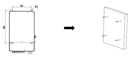
**Step 2**: Lift up the inverter and align the hole of the inverter with the expansion bolt, Fix the inverter on the wall.
