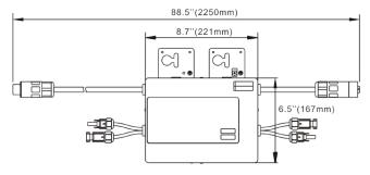
Our flagship product, the APsystems YC500A is a grid-tied microinverter with intelligent networking and monitoring systems to ensure maximum efficiency. Highly dependable and cost effective, the YC500A can accommodate PV modules up to 365W with dual MPPT but is ideally suited for modules from 280 to 310W. Half the inverters and half the installation means real cost savings for residential and commercial customers.
