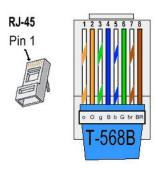
If needed, the network cable should be made like that diagram. But the cable should be made following the definition on battery side. If available, use a LAN cable tester to check whether the cable is faulty.
