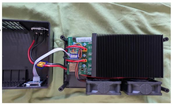
Disconnect the 2 DC XT connectors and the 2 FAN connectors (all in BLUE)
